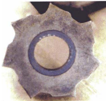
Fine abrasive particles can result in a fine matte finish such as that shown here.
