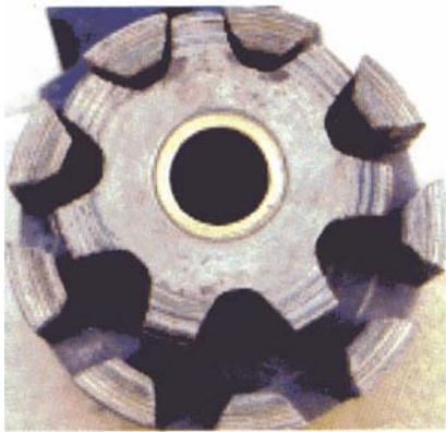
Large abrasive particles tend to leave score marks such as those shown here.
